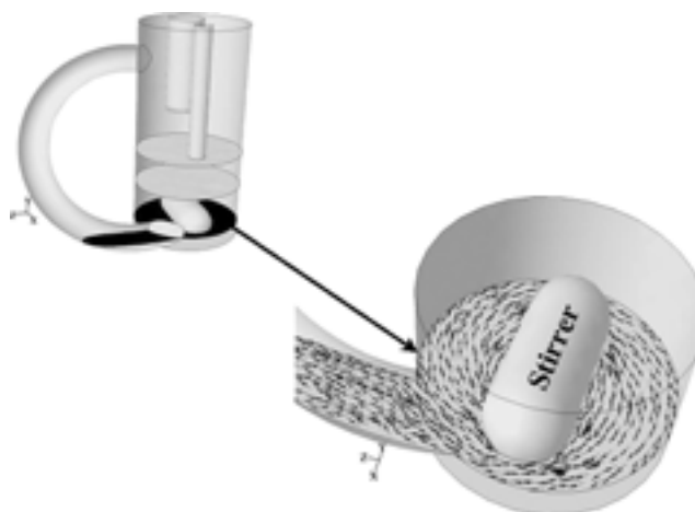
Fig. 3. Vector plots showing the velocity fields obtained at the bottom of the cell with clockwise rotation.
